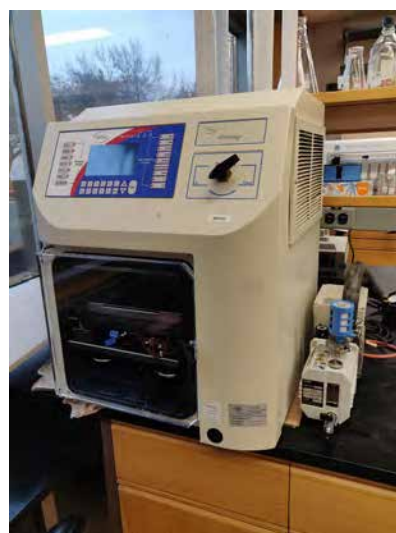
Lyophilizer, which is used to remove water from samples so it can be used in various procedures.
