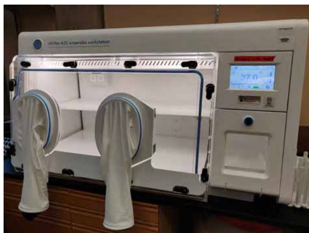
Anaerobic chamber which allows researchers to grow bacteria under zero-oxygen conditions to mimic the inside of our intestines.
